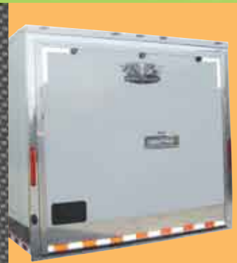
Single Handle Recessed Latch Ramp Door with L.E.D. Taillights.
