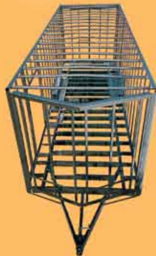
All Vintage Trailers are Constructed 16" on Center with 1" x 1-1/2" Box Tube Sidewalls.
